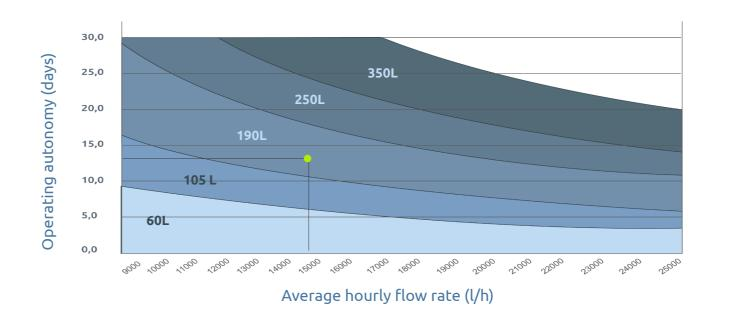
«Example: for an average flow rate of 15000l/h and an autonomy of 13 days, the volume of your tank will be 190L for the GRAVIKIT 30D90»
