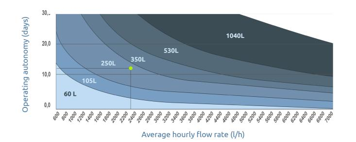
«Example: for an average flow rate of 2300l/h and an autonomy of 10 days, the volume of your tank will be 250 L for the GRAVIKIT 8D50»
