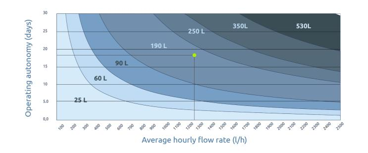
«Example: for an average flow rate of 1250l/h and an autonomy of 18 days, the volume of your tank will be 190 L for the GRAVIKIT 3D25».
