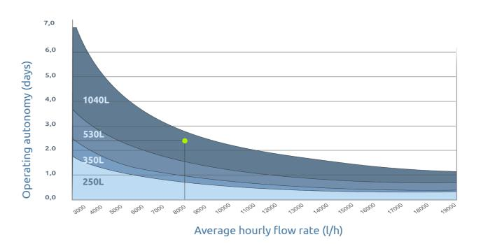
«Example: for an average flow rate of 8000l/h and an autonomy of 10 days, the volume of your tank will be 1040 L for the GRAVIKIT 20D63»
